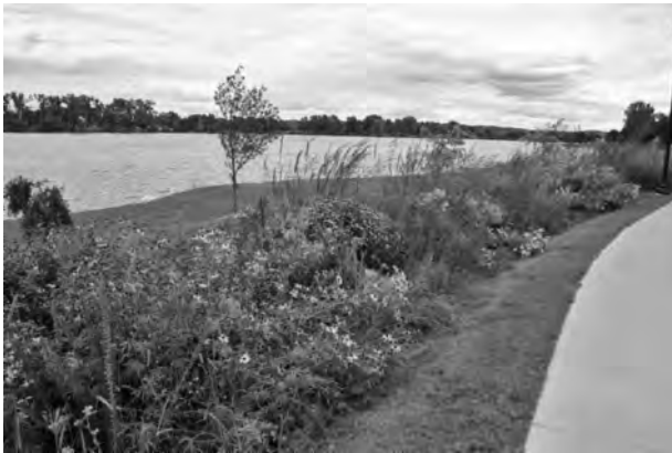
Figure 4-21 Interest in rain gardens continues as municipalities, landscape managers, and others look for sustainable ways to manage storm water. This rain garden is an effective way to prevent runoff into the nearby river.
