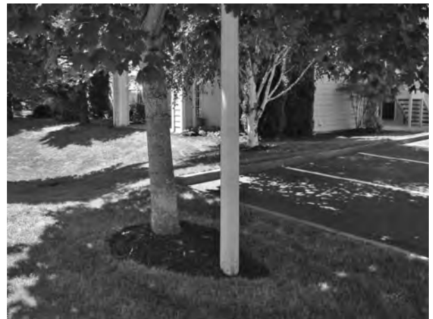
Figure 4-13 Clearly, the light (on the right) is too close to the tree to be functional. This layout should never have been installed.
